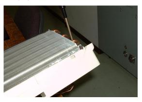
② Remove the screw (1) for the fan bearing cover.
